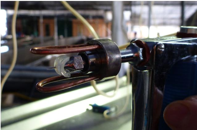
Picture 23: Needle guard is highly recommended
